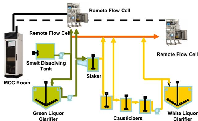
Figure 1A. Schematic illustration of the FT-NIR installation for smelt dissolving tank measurements.
