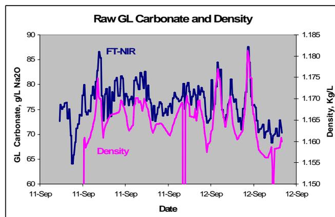
Figure 5. FT-NIR GL carbonate plotted with green liquor density.
