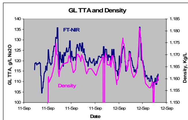
Figure 3. Dissolving tank FT-NIR TTA and dissolver density. The FT-NIR TTA is shown to correlate well with the density for this period.
