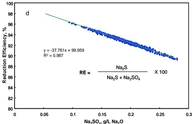
Figures 7a-d. Relationship between green liquor reduction efficiencies variations with chemical compositions: (a) sulphide, (b) thiosulphate, (c) sulphate with RE calculation including thio and (d) sulphate with RE calculation not including thio.
