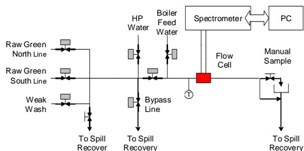
Figure 2. Typical sample line installation and valve hook up. Multiple samples can be tied into a sample tree and sequenced for sequential analyses with one flow cell. Each spectrometer can accommodate up to eight flow cells.
