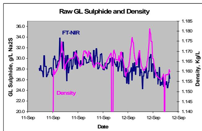
Figure 6. FT-NIR GL Sulphide concentrations with dissolver density.
