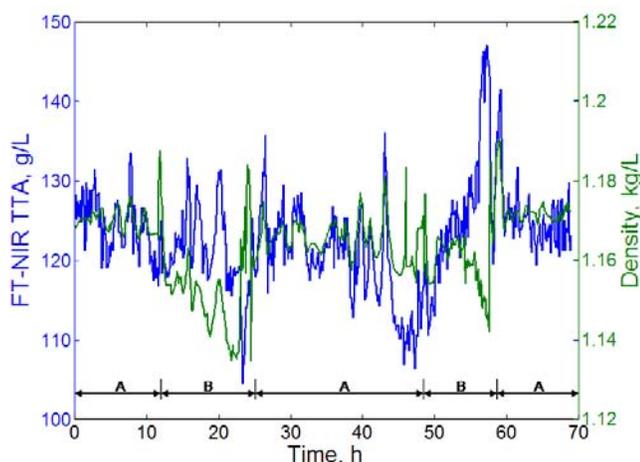
Figure 6. Comparing FT-NIR TTA (blue) results with dissolver density (green) meters. Period A and B refer to density meter readings on A and B transfer lines.
