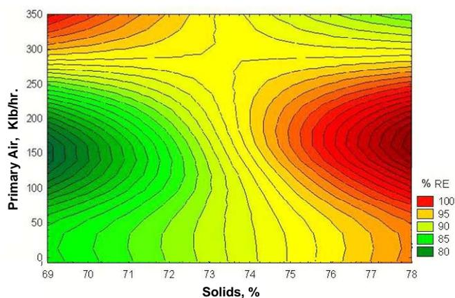
Figure 12. Contour plot relating primary air flow with black liquor solids content to green liquor reduction efficiency. Red indicates higher reduction efficiency.
